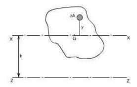
If 'ZZ' is any axis in the plane of cross-section and 'XX' is a parallel axis through the centroid G, of the cross-section, then
