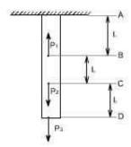
When either the axial force or the cross – sectional area varies continuously along the axis of the bar, then equation (1) is no longer suitable. Instead, the elongation can be found by considering a deferential element of a bar and then the equation (1) becomes
