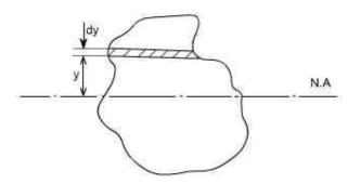
Consider any arbitrary a cross-section of beam, as shown above now the strain on a fibre at a distance 'y' from the N.A, is given by the expression
