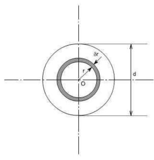
Consider any circular strip of thickness r located at a radius 'r'.
