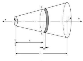
consider the above figure let  $r_1$  be the radius at the smaller end. Then at a X crosssection XX located at a distance x from the smaller end, the value of radius is equal to
