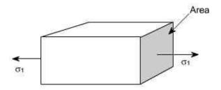
This is also known as uniaxial state of stress, because the stresses acts only in one direction however, such a state rarely exists, therefore we have biaxial and triaxial state of stresses where either the two mutually perpendicular normal stresses acts or three mutually perpendicular normal stresses acts as shown in the figures below:
