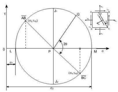
As we know that the circle represents all possible states of normal and shear stress on any plane through a stresses point in a material. Further we have seen that the co-ordinates of the point 'Q' are seen to be the same as those derived from
