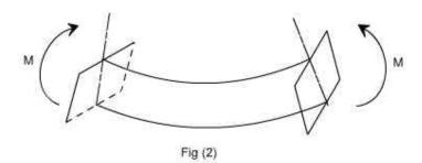
When a member is loaded in such a fashion it is said to be in <u>pure bending.</u> The examples of pure bending have been indicated in EX 1 and EX 2 as shown below:
