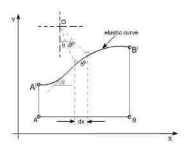
It may be noted that d is an angle subtended by an arc element ds and M is the bending moment to which this element is subjected.
