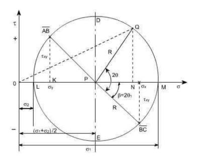
Consider any point Q on the circumference of the circle, such that PQ makes an angle 2 with BC, and drop a perpendicular from Q to meet the s axis at N.Then OQ represents the resultant stress on the plane an angle  $\,$  to BC. Here we have assumed that  $\,_{\rm X}$
