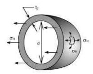
Because of the symmetry of the sphere the stresses set up owing to internal pressure will be two mutually perpendicular hoops or circumferential stresses of equal values. Again the radial stresses are neglected in comparison to the hoop stresses as with this cylinder having thickness to diametre less than 1:20.
